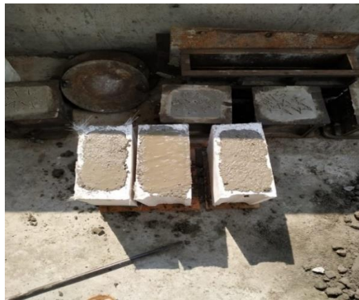
Figure-5. GFRG block filled with RAC
