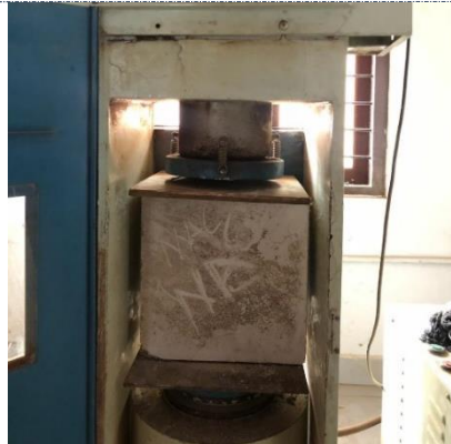
Figure-4. Test on GFRG filled with NAC
